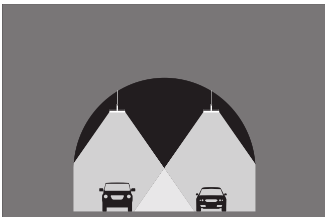
Two-way tunnel simulation with double light point, one for each carriageway
