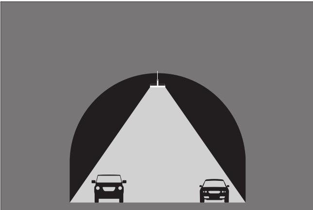
Two-way tunnel simulation with single central light point
