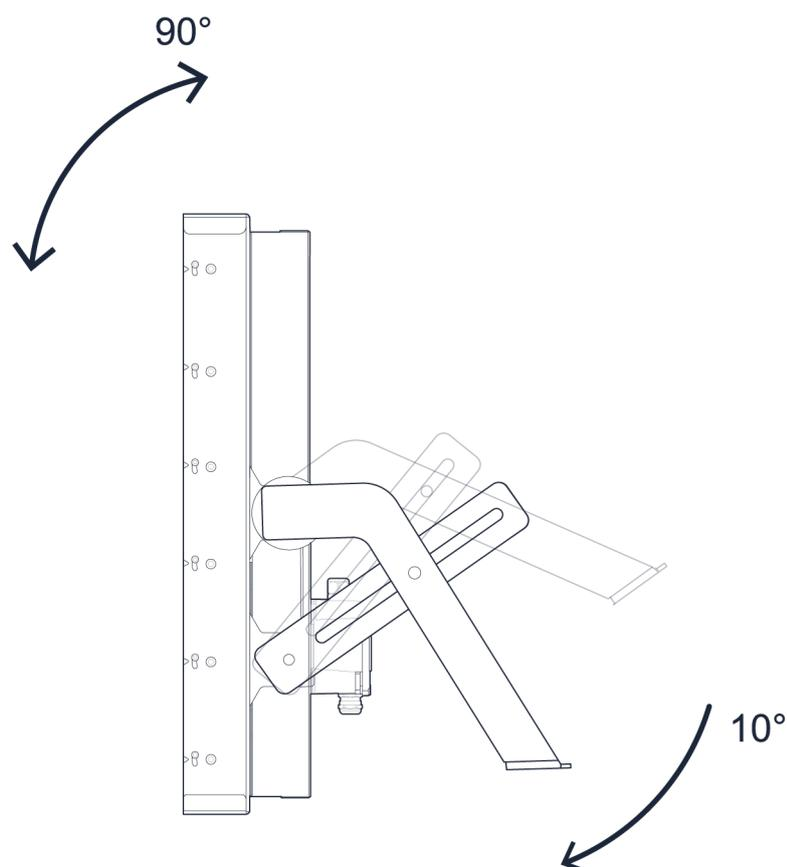
Wide mounting bracket can rotate up to 10° allowing the product to adjust the luminaire to the installation conditions (walls, parapets, balconies...). With this configuration the body luminaire can rotate up to 90°
