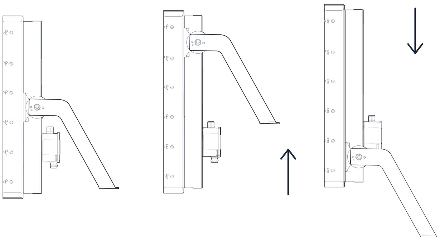
Different modes of connection of the bracket. It is in use in 4 modules, 5 modules, 6 modules, 12 modules
