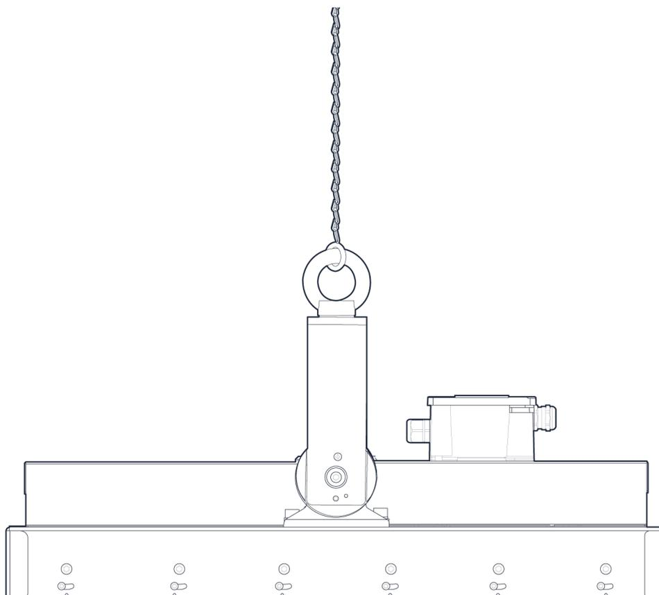
For installation in the pendant mode, the installation bracket must be installed in the middle of luminaire
