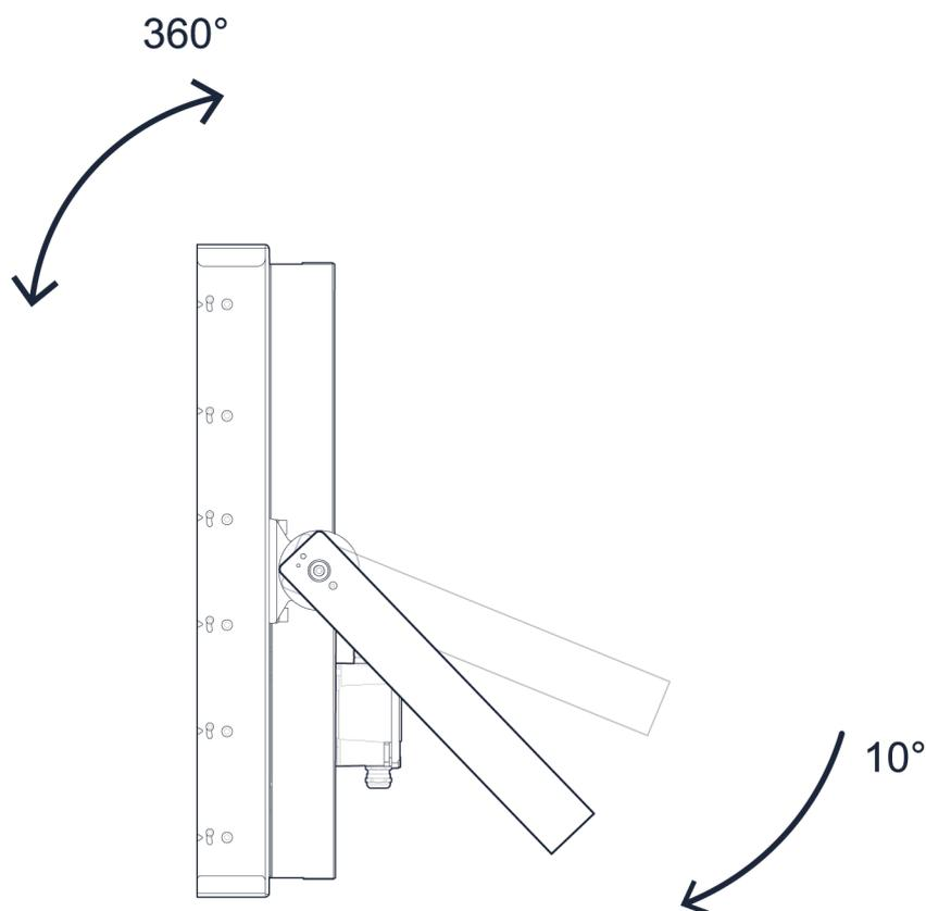
Simple long mounting bracket can rotate up to 10° allowing the product to adjust the luminaire to the installation conditions (walls, parapets, balconies...). With this configuration the body luminaire can rotate up to 360°
