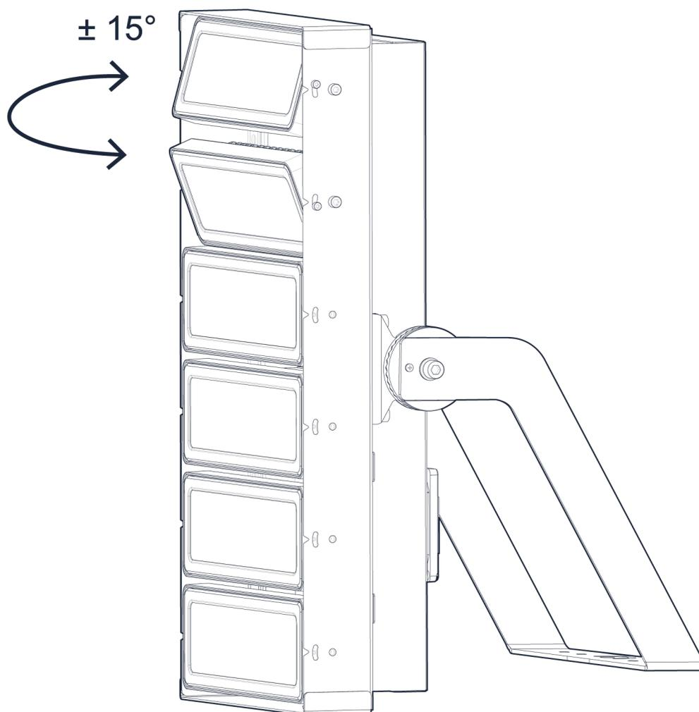
Modules can rotate in the horizontal axis by  $15^\circ$  upwards or downwards
