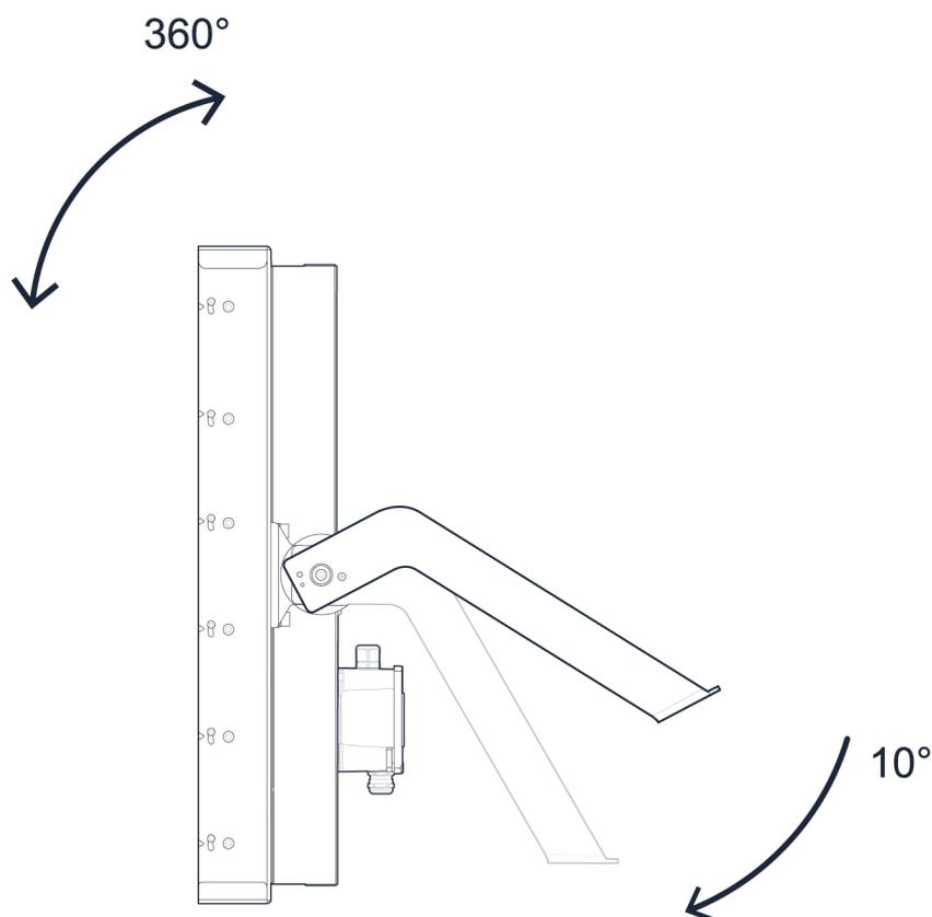
Oblique long mounting bracket can rotate up to 10° allowing the product to adjust the luminaire to the installation conditions (walls, parapets, balconies...). With this configuration the body luminaire can rotate up to 360°
