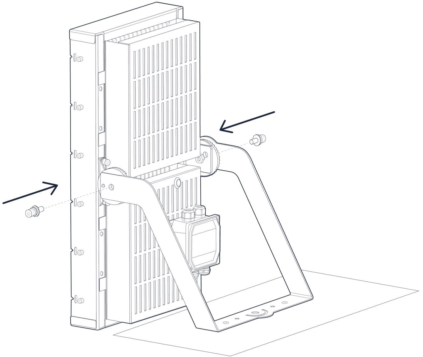
Loosen the gland, pass the cable through it and direct the cable into the floodlight. Installing the luminaire to body M8 allen screws then, fasten the installation base when adjusting the desired angle
